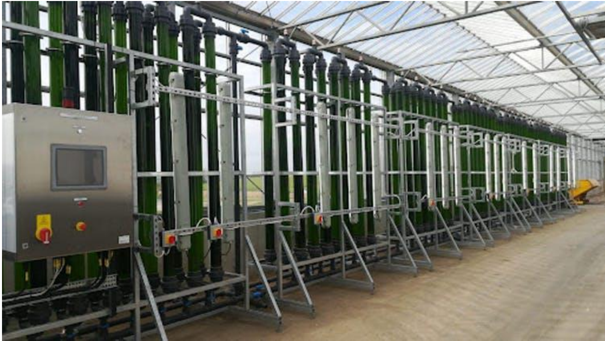
The 7,000 L Algal photobioreactor, constructed in a heated greenhouse at Langage-AD in Devon. Photo: Claudio Fuentes-Grünwald, Author provided
